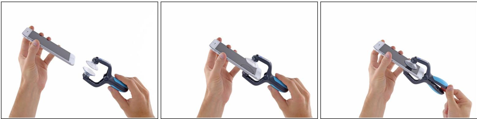
**i** The next two steps demonstrate using the [iSclack](#), a great tool for safely opening the iPhone 6 Plus that we recommend for anyone doing more than one repair. **If you aren't using the iSclack, skip down two steps.**
